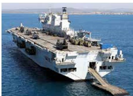
Custom hull access doors of all types are available including sliding, roller gate, folding, and hinged. Depending on type, these can be supplied as watertight or weathertight. Special consideration is taken to ensure flexibility for various naval operating requirements such as RCS minimisation and the rapid deployment of equipment.
