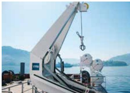
All TTS winches are designed to meet hydraulic and electrical class requirements. Our unique self-contained models have electro-hydraulic drives with built-in power packs, reducing maintenance costs and minimising risk of oil spill and damage. TTS davits are available in a number of custom configurations – such as A-frame, swing-out and telescopic – all designed to meet the latest SOLAS requirements.
