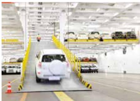
TTS expertise in vehicle decks and ramps has made us a global leader and the first choice of the world's largest vessel operators. A number of governments have entrusted TTS to provide custom solutions in order to enhance flexibility and operational effectiveness of their vessels. Requirements such as water/gas tightness, adjustable heights and design for heavy loads can be accommodated.
